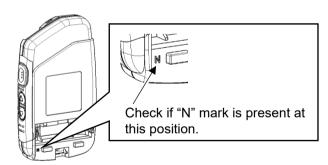
The back of the meter (with the battery cover removed)
